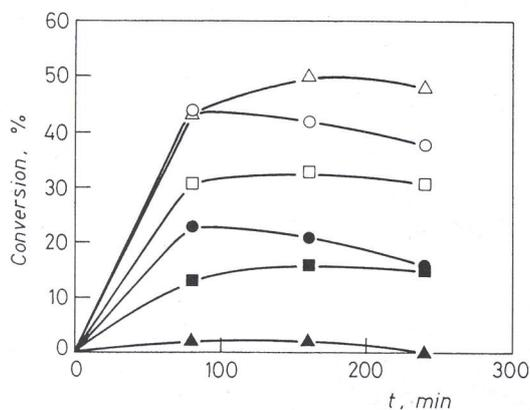
**Fig. 3.** Solvent-naphtha hydrogenation with 1.5 wt % catalyst E at 80 bar. Evolution of indene and coumarone conversion with time for different reaction temperatures: (Δ) indene, 200°C; (□) indene, 250°C; (○) indene, 300°C; (▲) coumarone, 200°C; (■) coumarone, 250°C; (○) coumarone, 300°C.
