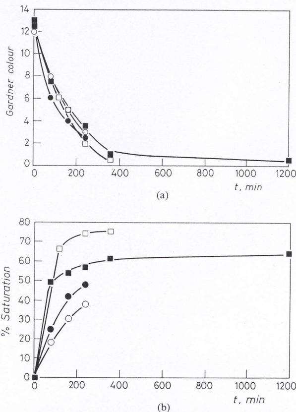
Fig. 1. Evolution of resin Gardner colour (a) and saturation (b) with reaction time for hydrogenation with 1.5 wt % catalyst E at different reaction conditions: (○) 250°C, 40 bar; (●) 250°C, 80 bar; (■) 250°C, 120 bar; (□) 300°C, 120 bar.
