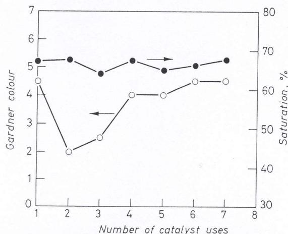
**Fig. 4.** Evolution of catalyst activity with successive uses. Indene-coumarone resins colour and saturation after hydrogenation with 3 wt % catalyst F (extrusions), at 250°C and 120 bar for 4 h, vs number of successive catalyst uses.
