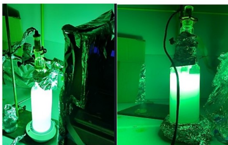
Figure ST2: 9.34 \text{ kW m}^{-2} at 4 cm medium-pressure mercury lamp (Novalight TQ150) used for the protocol.
